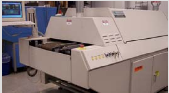
Conceptronics 60 reflow oven is qualified for fine-pitch, double-sided, lead-free (RoHS) boards.
