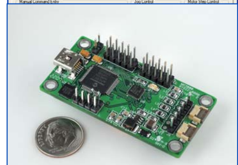
Closed-loop controller for 2 motors
